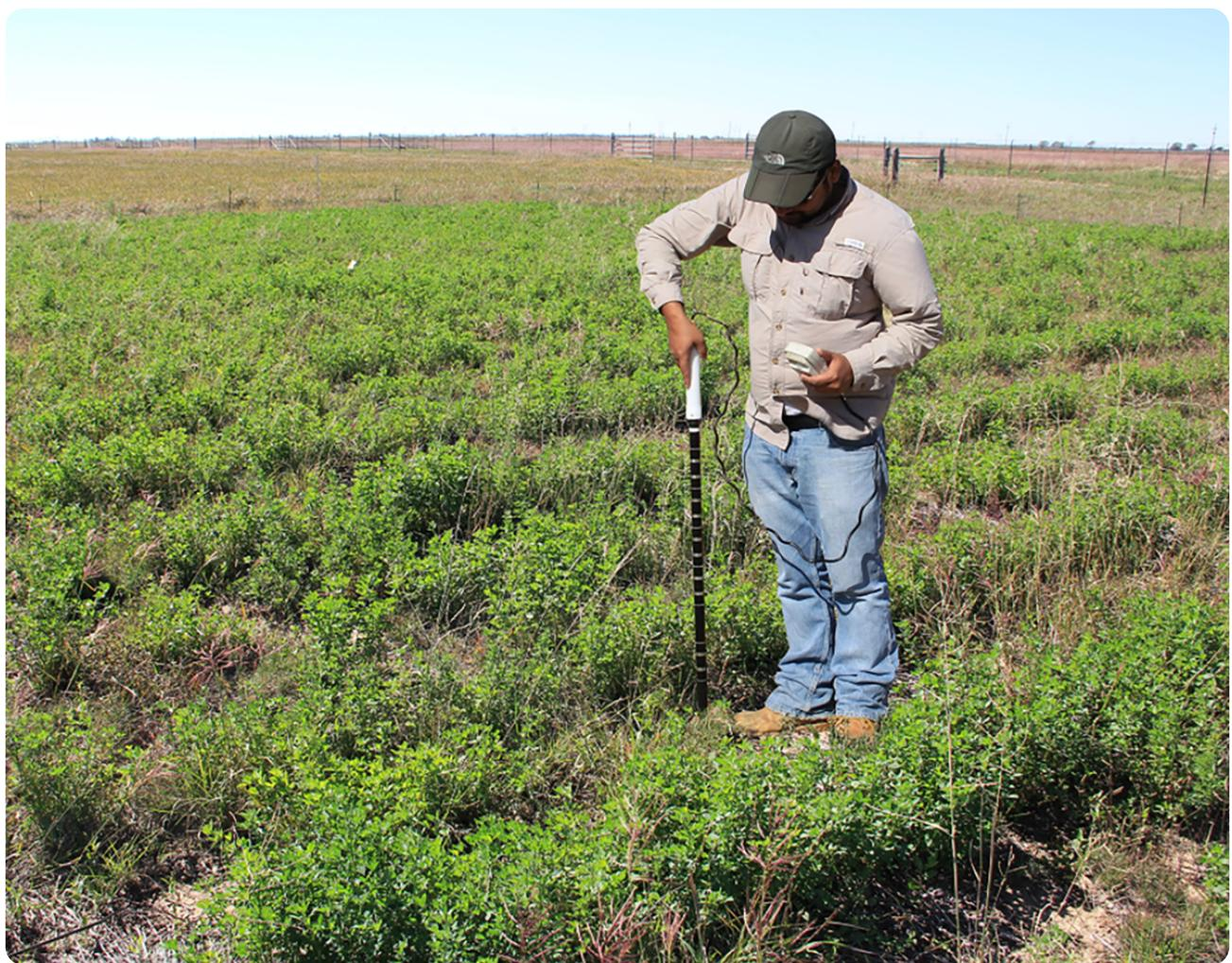
*Researcher measuring soil volumetric water content using a portable PR2 capacitance probe between two alfalfa rows in Texas.*
