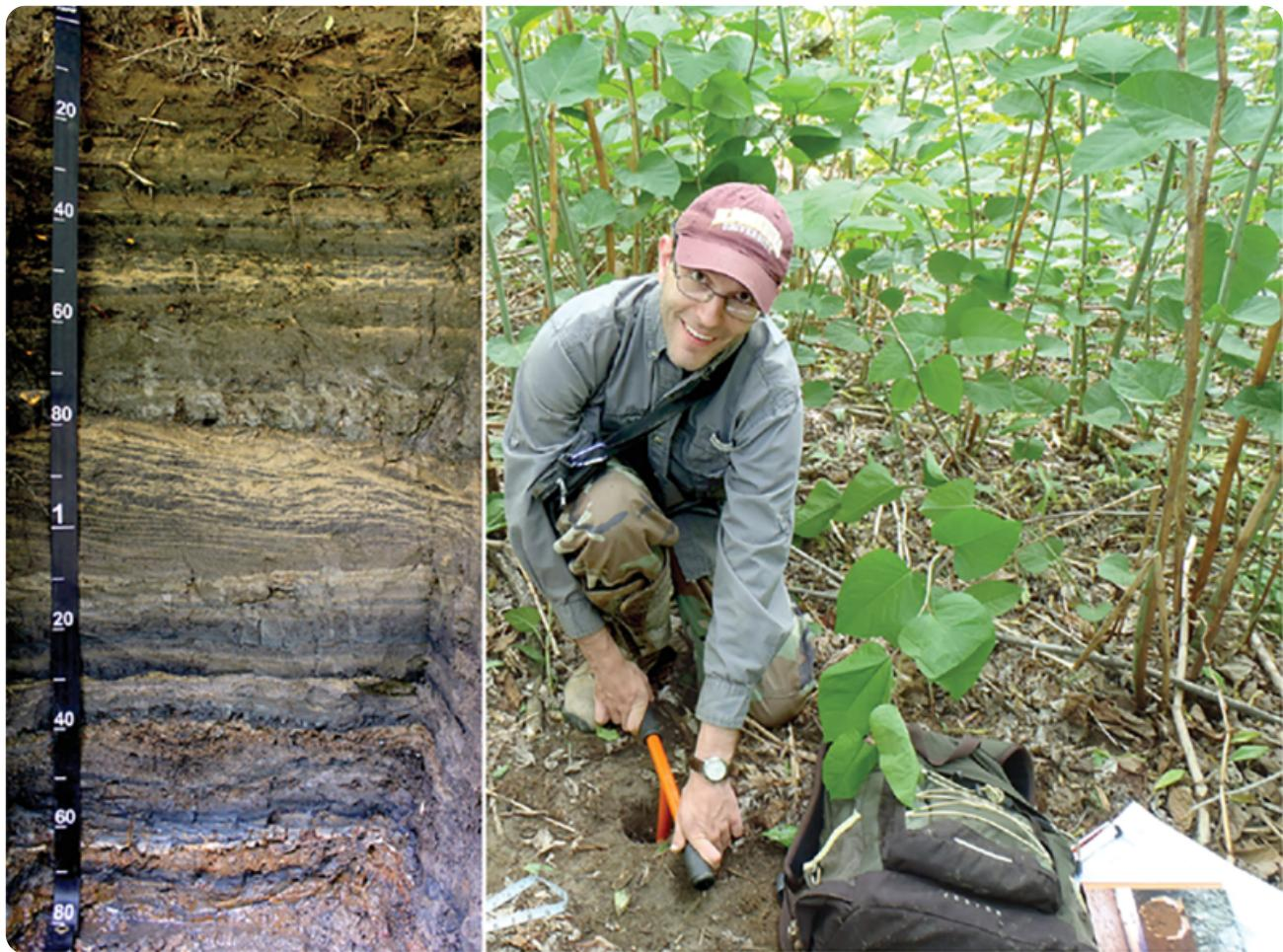
*Left: Stratified alluvial anthracite coal in the floodplain of the North Branch of the Susquehanna River (tape scale in cm). Right: North Carolina State University Assistant Professor Matt Ricker uses a hand auger to collect deep alluvial soil samples. Photo*
