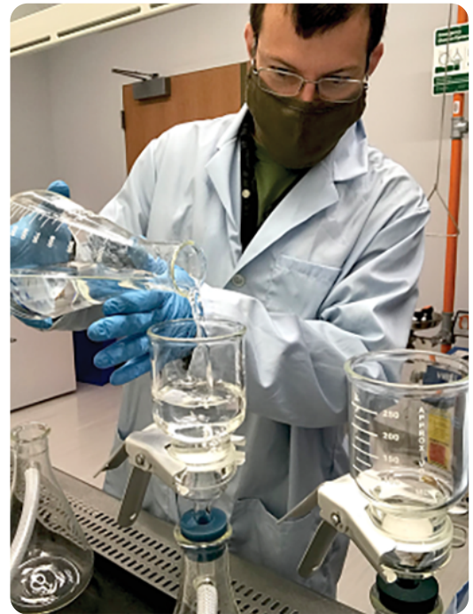
Penn State lab technician Bill Clees filters a wastewater effluent sample that will be analyzed for pharmaceuticals. Photo by Heather Preisendanz.
