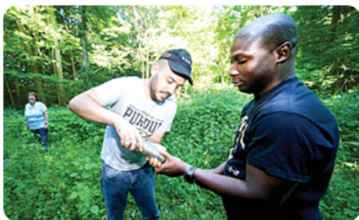
Soil coring for transport studies of per- and polyfluoroalkyl substances
