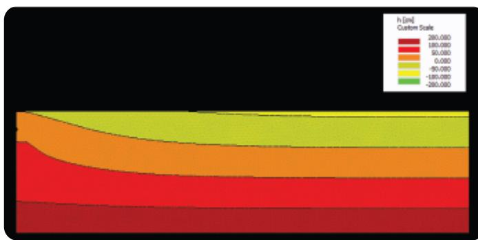
*Steady-state pressure heads ( $h$ ) after wastewater addition for a soil in the moderate hydraulic conductivity class. Wastewater was introduced through the pipe in the gravel-filled trench (notch in upper left). X dimension = 1,500 cm; Z dimension = 200 cm. Vertical exaggeration is 2X.*
