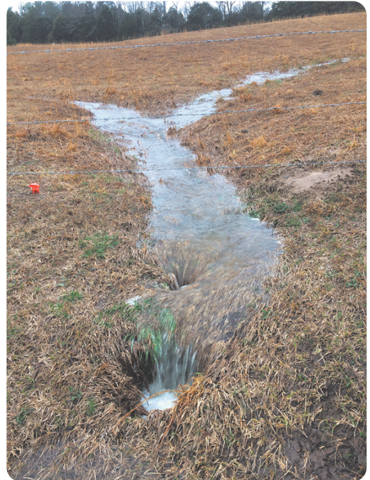
Storm runoff from two branches of a catchment in Goodwin Creek Experimental Watershed, MS is intercepted by soil pipe collapse flute holes and diverted into subsurface flow through a soil pipe.
