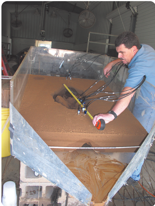
Alan Hudspeth measuring the pipe collapse following an experiment with flow through a soil pipe that was initially 10 mm in diameter under a constant head inflow condition.
