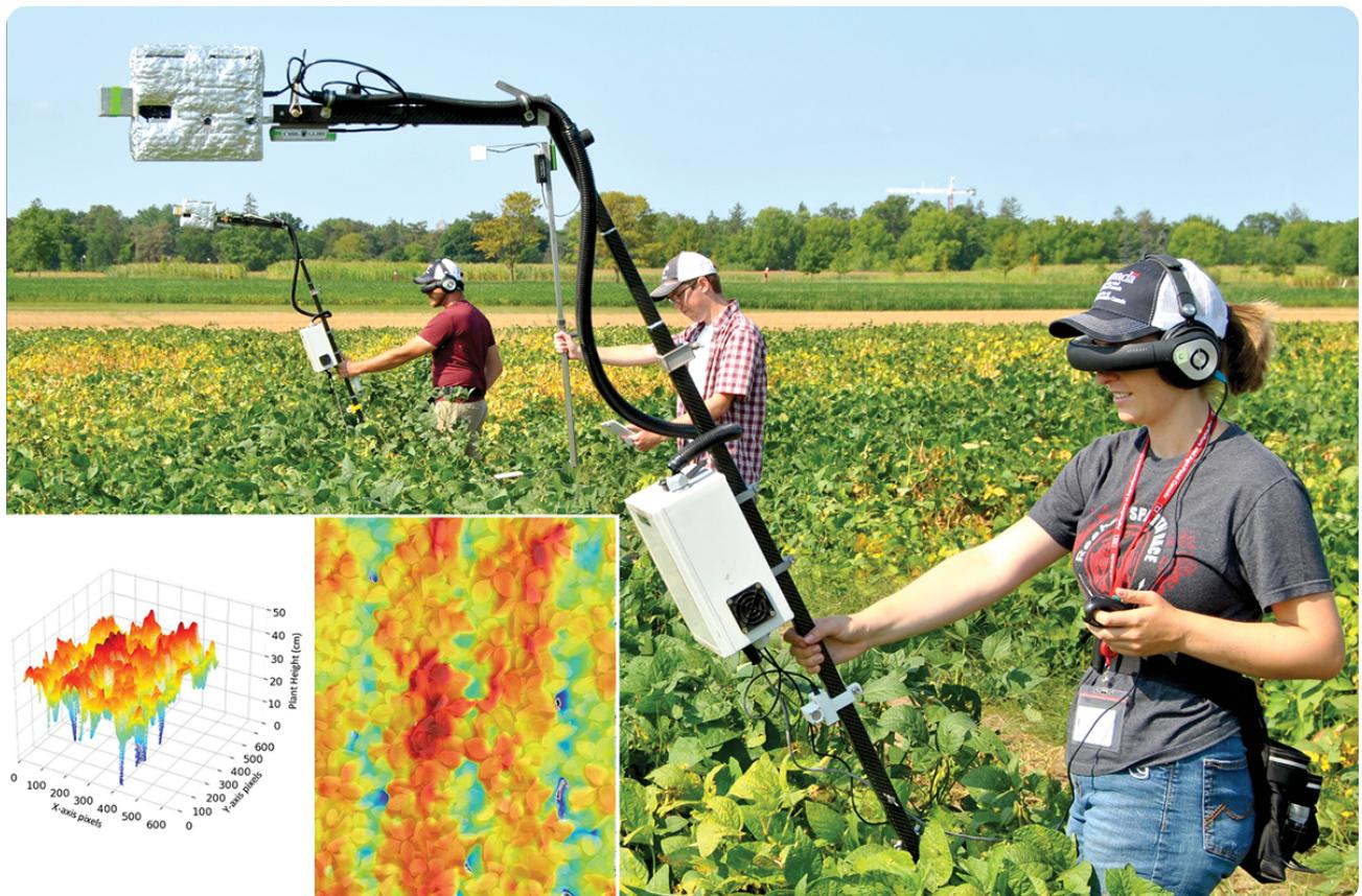
*The D415 camera is mounted anterior to the heat reflective wrapped RGB and infrared camera housing on the PlotCam. The HeightStick is a single-point LIDAR aimed down to a vertically movable paddle set at the top of the canopy; data are stored on a tablet via Bluetooth. Inset: A 3D plot of 480- x 640-pixel soybean canopy heights and a 2D overlay of the heights over a nadir RGB image at the beginning of flowering. Courtesy of Soybean*
