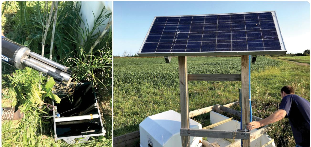
*Left: Deployment of a YSI EXO 3 sonde in a drainage water management control structure. Right: Researcher at a USDA-ARS edge-of-field monitoring station. Photos courtesy of Saeid Nazari.*
