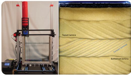
*Left: A Queen's University research team modified this 3D printer so that it could dispense sand. Right: An example of a heterogeneous sand pack created by the modified 3D printer. Photos by Mitchell Davidson.*
