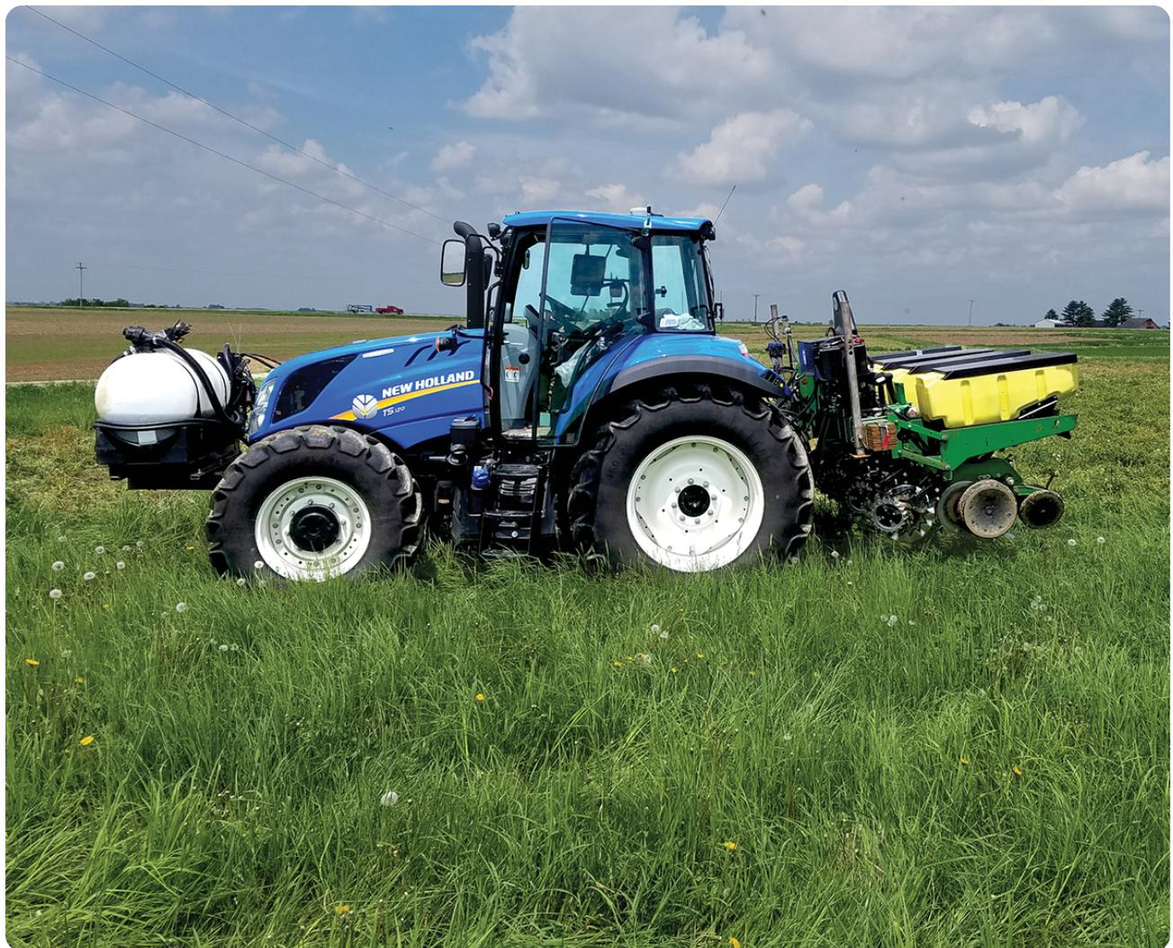
*Research planter equipped with hydraulic row-unit downforce, various closing-wheel systems, and variable-rate starter fertilizer. Utilizing these technologies, planting corn in no-till production systems can help with emergence depending on soil conditions. Photo by Brian Luck.*
