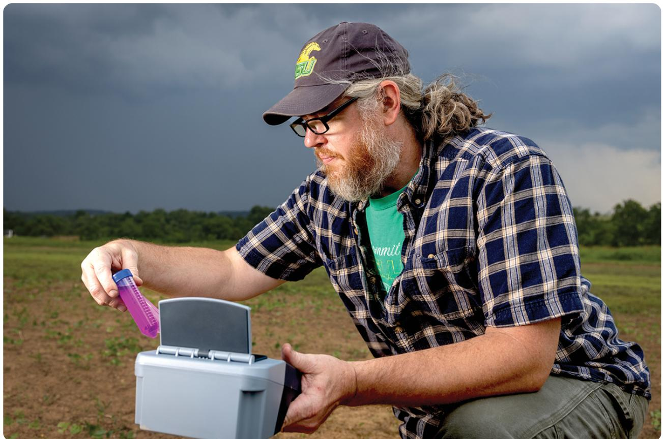
*Co-author Shawn Lucas gathers information on the soil carbon status of a field by analyzing permanganate oxidizable soil carbon. Modern handheld spectrophotometers make this rapid and practical method easy to incorporate into field assessment kits. Photo by Jonathan Palmer.*
