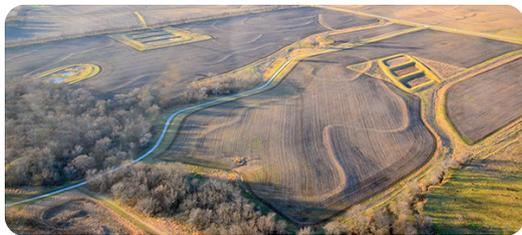
*Three constructed wetlands, each made up of three interconnected “cells,” at the Franklin Research and Demonstration Farm. Even one cell filtered significant amounts of nutrients from water coming from adjacent tile-drained farmland.
