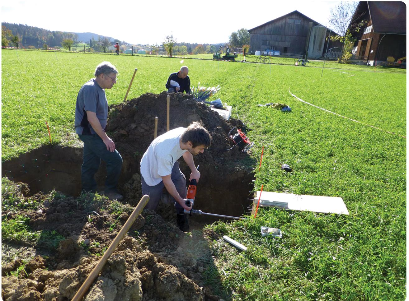
*Preparation for installation of soil-embedded sensors used for continuous in situ measurements of state variables. Photo courtesy of Agroscope.*
