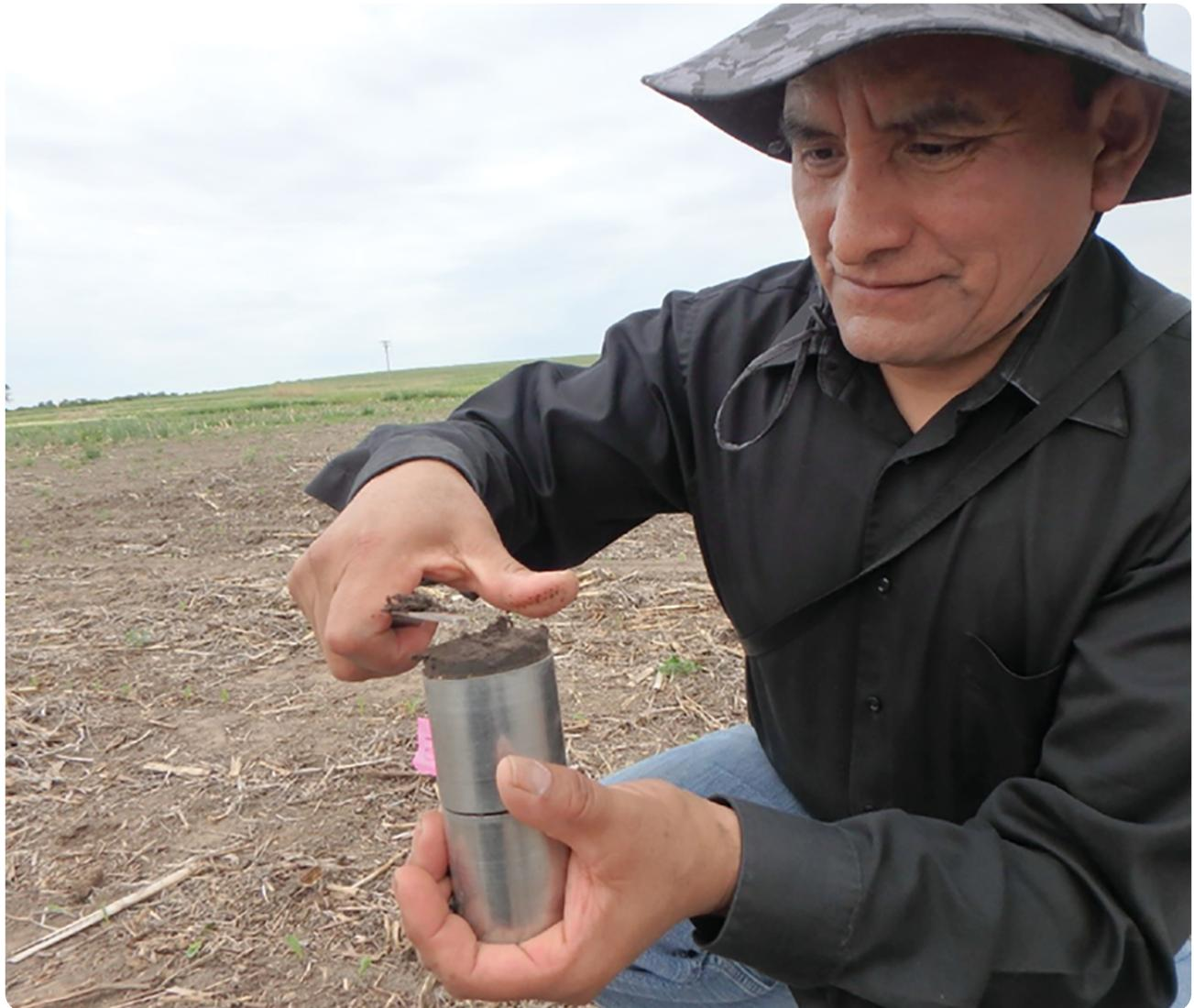
*Author Humberto Blanco collecting and trimming intact soil cores from field plots to determine soil bulk density required for computing soil organic C stock. Photo courtesy of*
