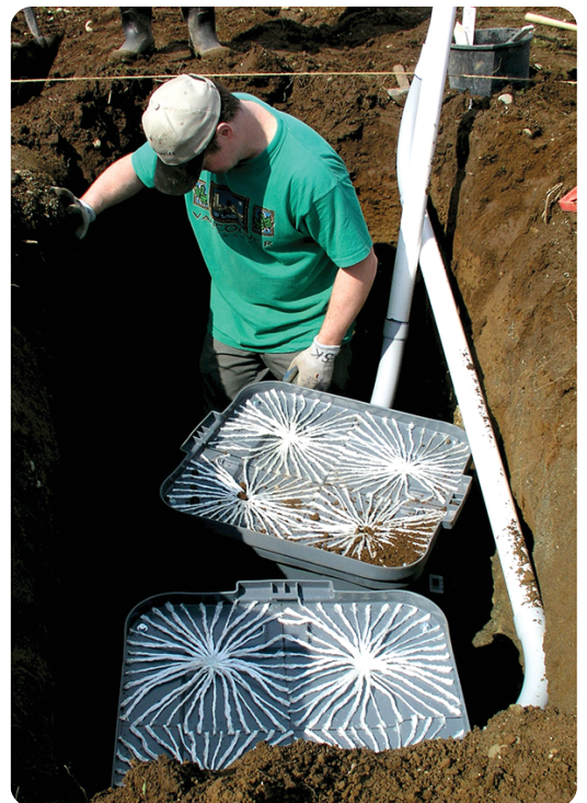
Scientist Tom Forge installs passive capillary wick samplers at the bottom of the rootzone prior to planting raspberry rows for the team’s multi-year experiment. The researchers dug 32 such holes to hold the instrumentation, which measured nitrate levels in water
