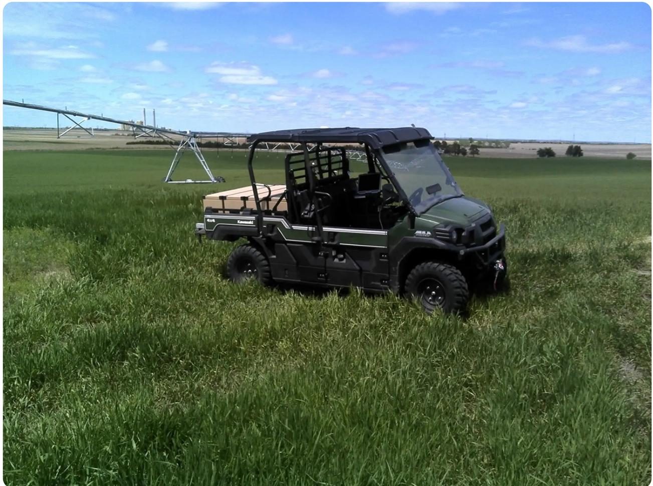
*A rover equipped with a cosmic-ray neutron sensing system for soil moisture mapping, representing one of several geophysical tools applied in agriculture. Photo courtesy of Trenton E. Franz, University of Nebraska-Lincoln.*
