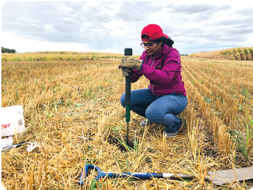
Jashanjeet Dhaliwal takes intact soil core samples to analyze soil physical and hydrological properties. Photo by Navdeep Singh.
