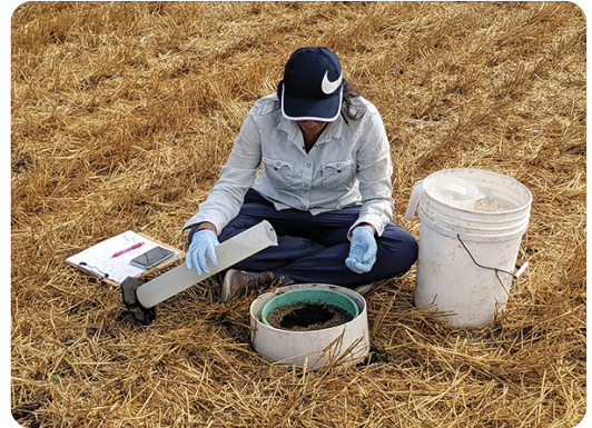
Jashanjeet Dhaliwal measures water infiltration with a double-ring infiltrometer. Photo by Udayakumar Sekaran.
