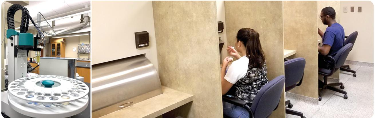
*Left: Sensory equipment in Sungeun Cho's lab at Auburn University. Right: A typical sensory trial setup where participants take samples provided through the small metal windows, taste, and rate samples in their individual cubicles. Photos by Sungeun Cho.*
