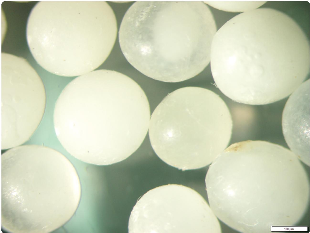
*Using microscopy to characterise the release stage of controlled-release fertilizers helped explain the effect of soil water on nitrogen release, highlighting the strengths of collaborating across disciplines. Photo by J.M. Poole.*
