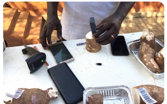
Enoch Webabzi, a graduate student at West Africa Center for Crop Improvement, uses a handheld spectrometer to analyze cassava roots at the Uganda National Crops Resources Research Institute. Photo by Jenna Hershberger.
