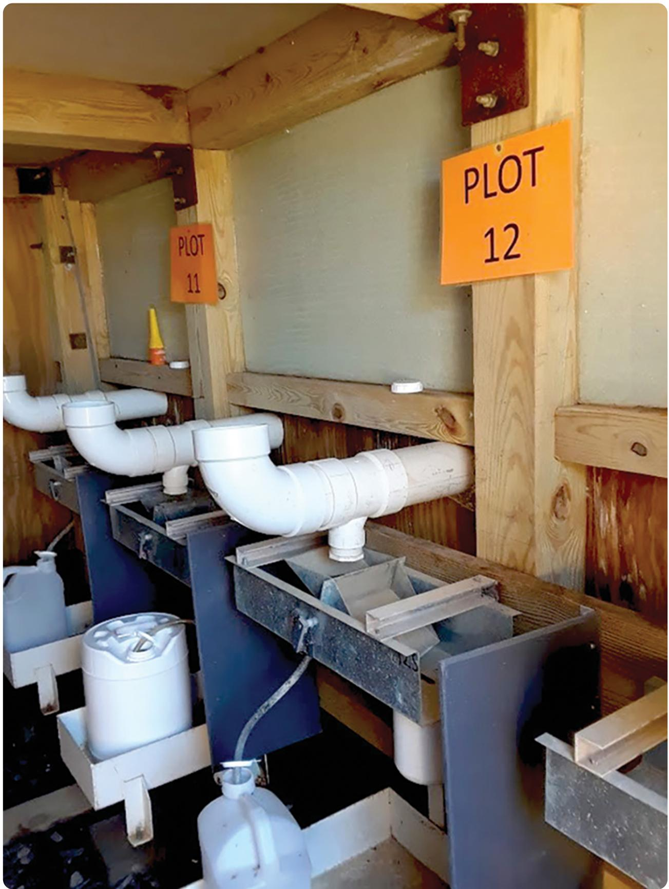
*Tipping buckets used to measure runoff from lysimeter plots. Photo by Sarah Frame.*
