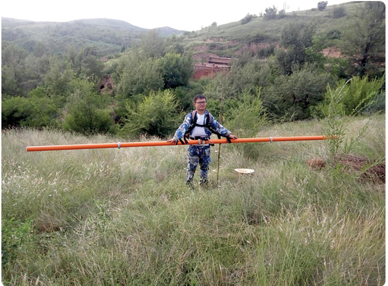
*Study author Qinbo Cheng carries an electromagnetic induction (EMI) explorer, which the team used to obtain soil bulk electrical conductivity data. Photo by Jiao Wang.*
