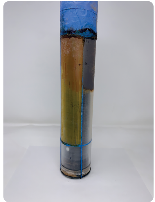
The IRIS tube after removal from the simulated wetland bucket system after 28 days. You can clearly see where microbes removed manganese and iron paint. Photo by Olivia LeFevre.
