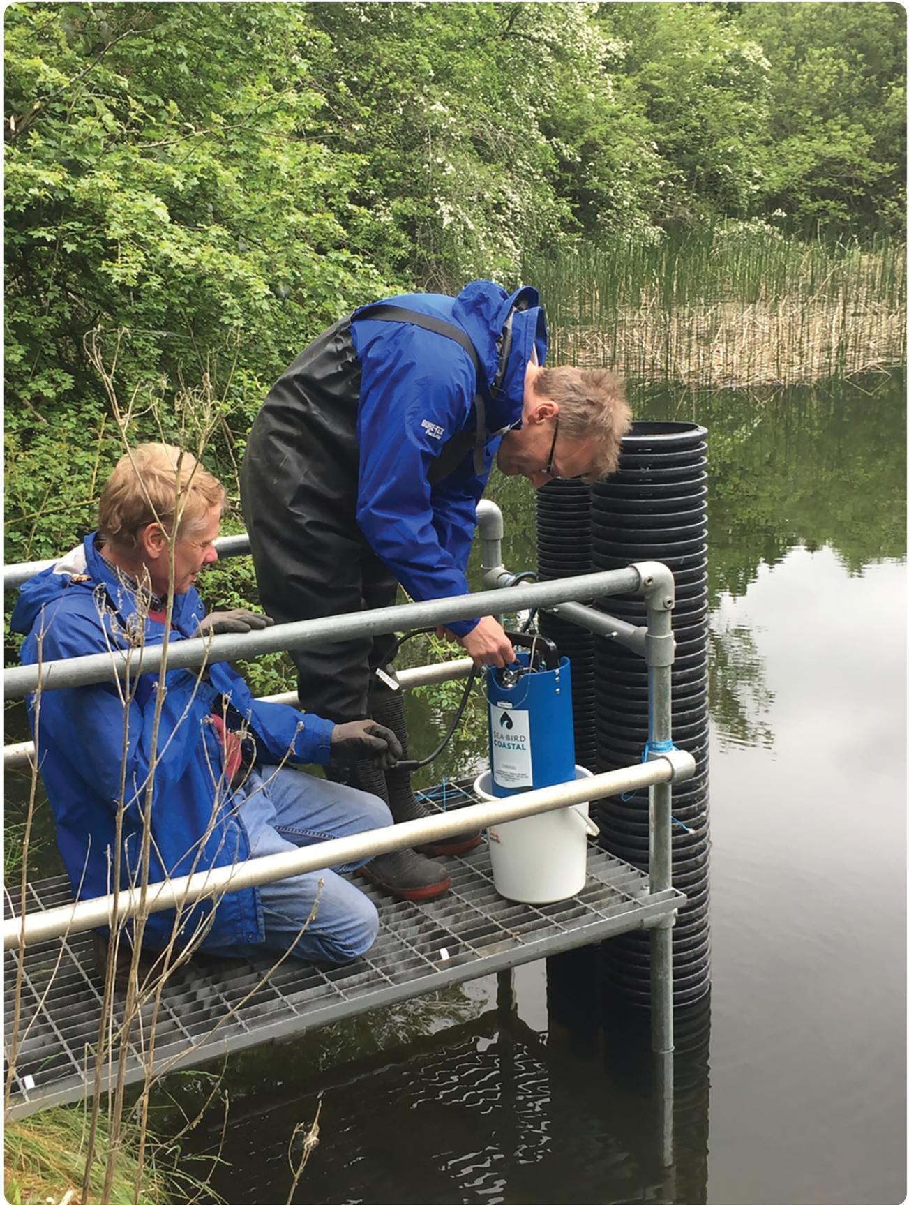
*Installing in situ nutrient sensors at the outlet of the wetland-pond system in Wytham, UK.
