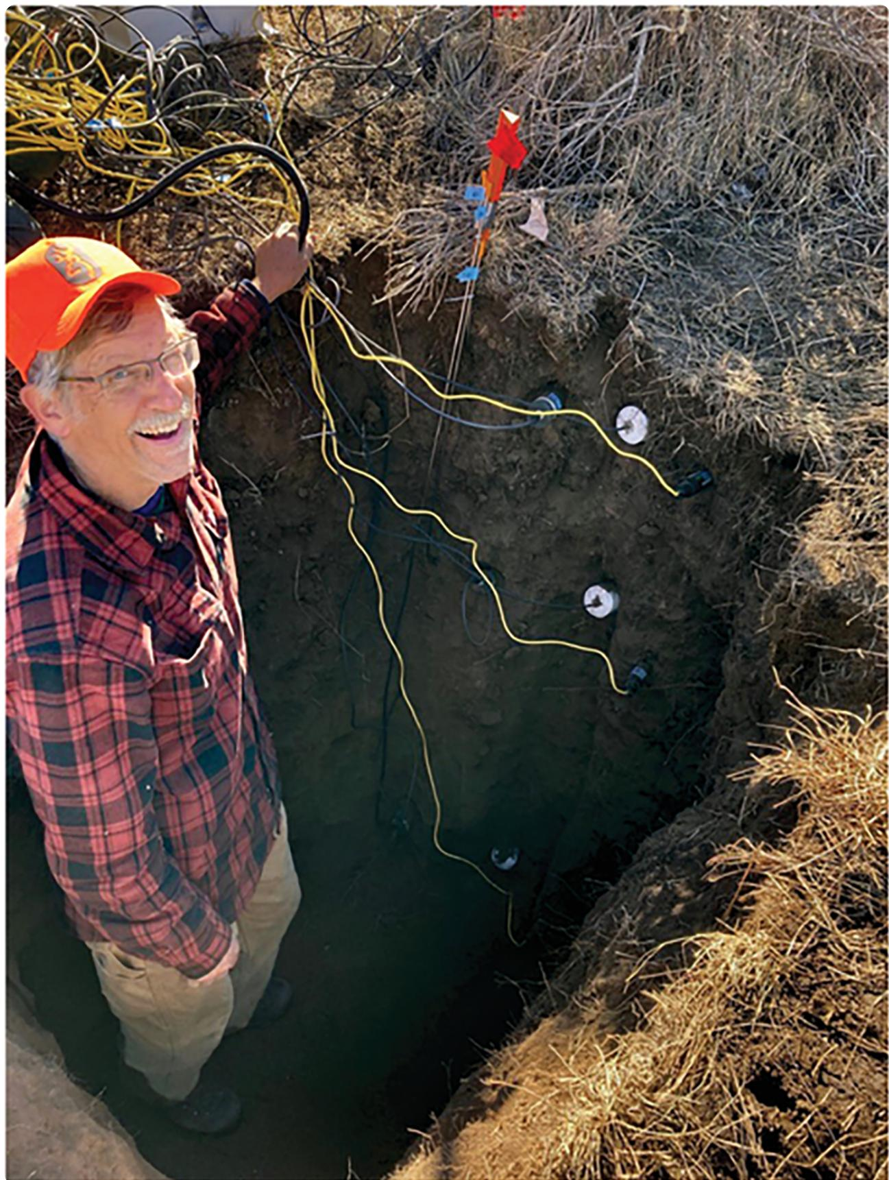
*Lead author Mark Seyfried in a soil pit instrumented for soil gas, water content, and temperature. Photo by Kathleen Lohse, Idaho State University.*
