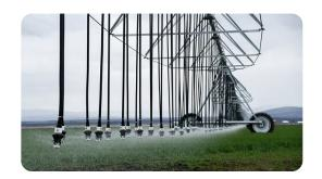
Research conducted at the CAFE site in Rupert, ID monitored differences in consumptive water use mid-elevation spray application (MESA) and low-elevation spray application (LESA) systems. Photo is not from the research site and is courtesy of NRCS Oregon. CC BY 2.0.
