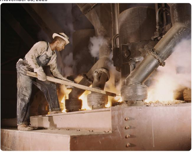
A large electric phosphate smelting furnace used to make elemental phosphorus in a TVA chemical plant near Muscle Shoals, AL in 1942. Source: United States Library of Congress.
