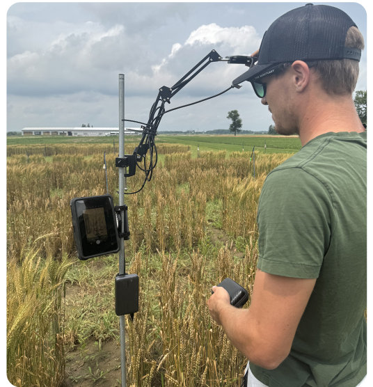
Riley McConachie using a cell phone connected to an external display to image wheat plots for Fusarium head blight evaluation.
