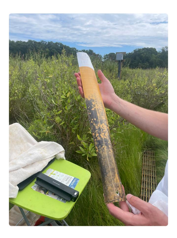
Indicator of Reduction in Soils (IRIS) film immediately after retrieval following 60-minute deployment in a tidal marsh soil. On the green table is a portable document scanner for collecting the IRIS image. Photo courtesy of Jocelyn Wardrup, UMD ENST.
