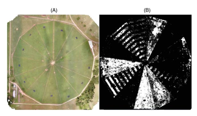
The above images illustrate precision agriculture in action. Left: A drone image of a field in north Florida. Right: A map of weeds gen- erated by an artificial intelligence algorithm that supports weed management in that same field. Using these tools to identify un- desirable plants for precision herbicide spraying saves labor and costs. Images by University of Florida–NFREC, Marianna.
