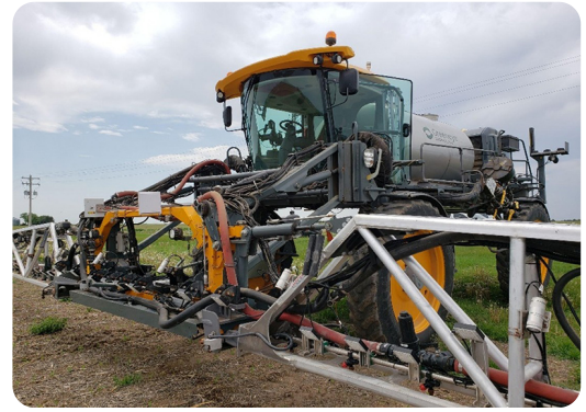
Figure 1. Greeneye Technology's precision sprayer used in this study.
