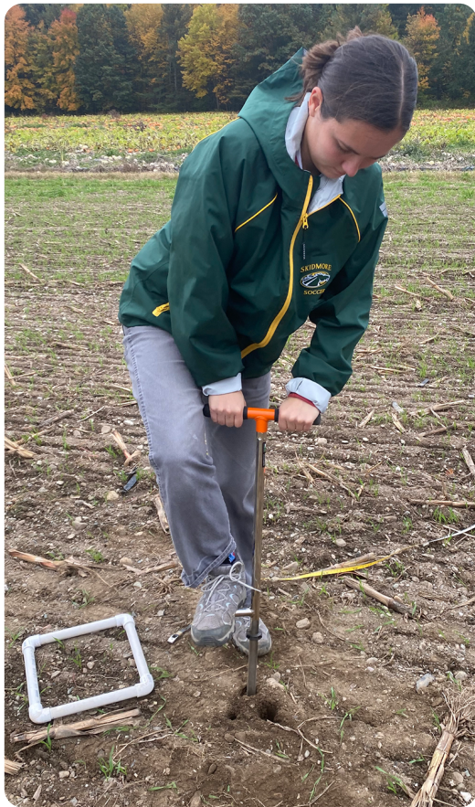
Direct measurement of SOC usually involves gathering soil samples and analyzing them using dry combustion methods. Photo by Kelsey Jensen.
