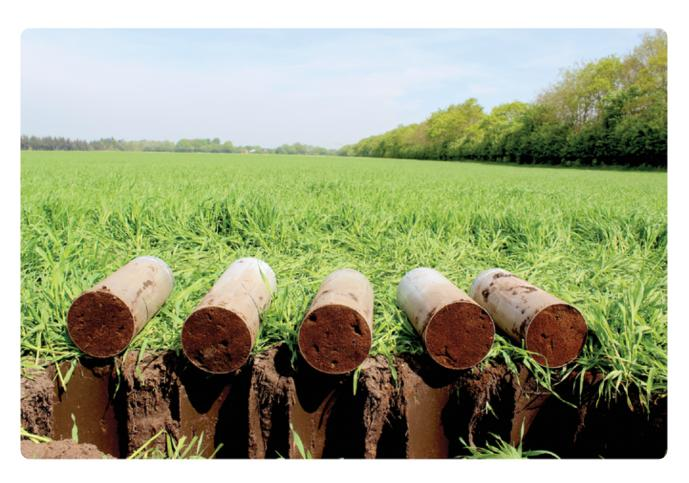
Researchers conducted an outdoor column study to compare the behavior of bromide in arable topsoil to control columns contain- ing sand and fine gravel. Photo by GEUS/Christian Albers.
