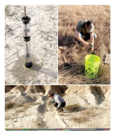
Clockwise from top: A mini disk infiltrometer measures infiltration of water into soil in the disturbed area, Texas A&M University grad- uate student Parker Murphree collects soil
