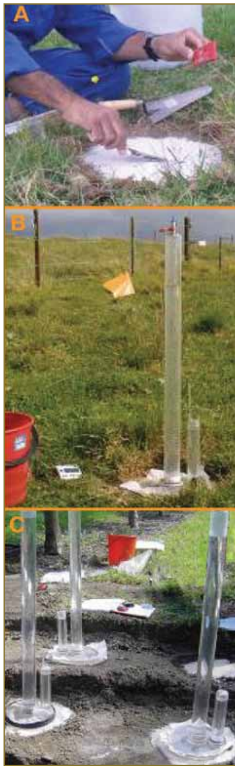
Fig. 2. The use of tension infiltrometers in the field. (A) Preparation of the contact sand as the infiltration surface atop the undisturbed soil. (B) Measurement of the infiltration rate at the surface. (C) Multiple and simultaneous measurement of infiltration rates at several depths in a soil profile.
