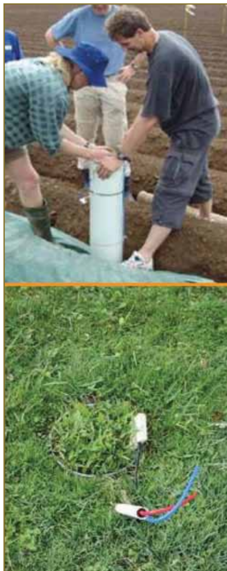
Fig. 4. The use of water-flux meters in the field. (Upper) Installation of a water-flux meter under potatoes. (Lower) A water-flux meter under pasture. The protruding tubes are for the calibration of the tipping spoon (light-colored tube) and the extraction of the soil solution (darker tube). Additionally, a CS616 soil moisture sensor was installed to measure the soil's water content (see the chapter on bulk density in this volume, Logsdon et al., 2008).
